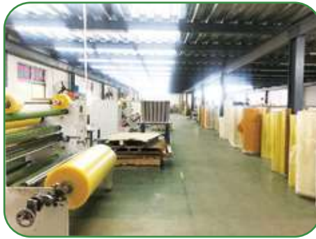
Jumbo rolls ready for converting
